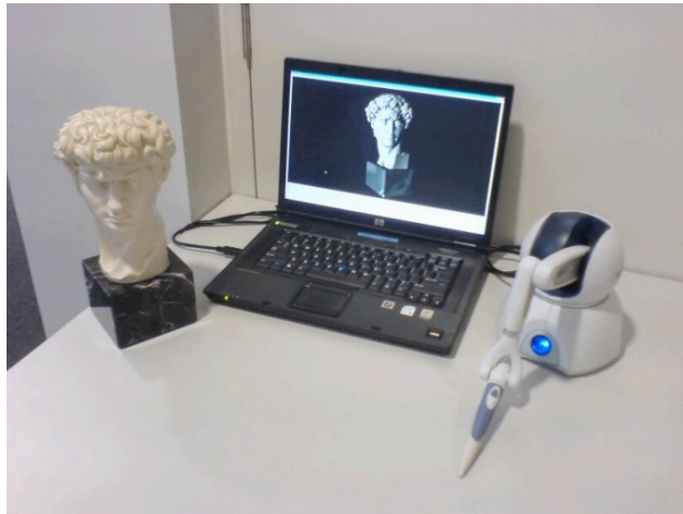
Figure 3: Physical and virtual sculpture with haptic device
